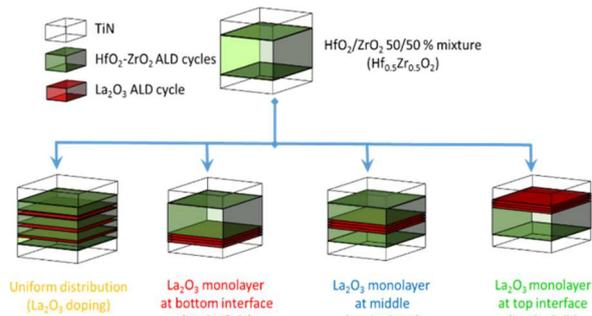
A LaO<sub>x</sub> monolayer (about 0.5 nm LaO<sub>x</sub>) showed the highest pristine remanent polarization values and low wake-up effects compared to the uniformly mixed case. Looking at the best position of the LaO<sub>x</sub> monolayer, the interface between the bottom TiN electrode and HfZrO<sub>4</sub> indicated lower fatigue. This result can be nicely seen as a clear cycling improvement with almost no wake-up effect in relation to the undoped and mixed doped case.
