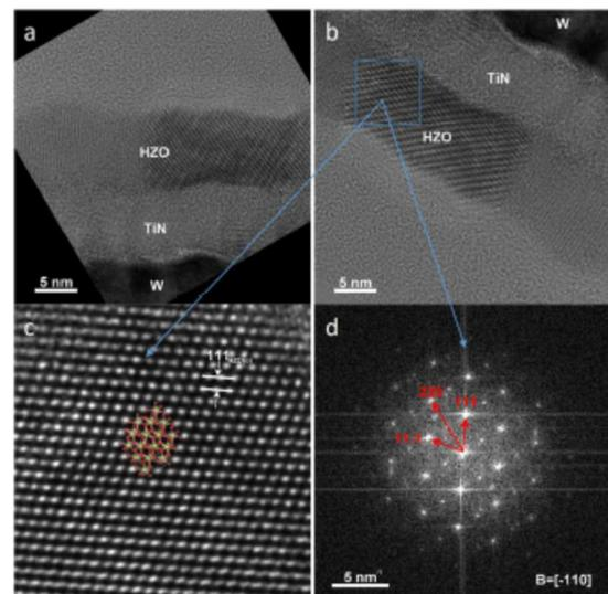
As an example, very good results were obtained for sample with the composition Al<sub>2</sub>O<sub>3</sub>/HZO/TiN/W/Si, in which the orthorhombic phase appears to be dominant, as revealed by TEM analysis.
