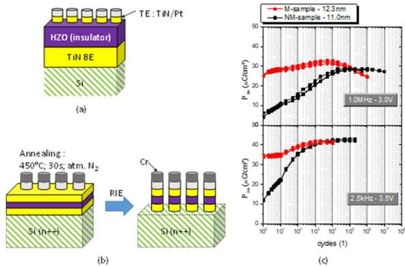
The two different structures realized have performances among the best in sputtering, but their behaviours are completely different. Mainly, the mesa structure presents a significantly reduced wake-up effect but a lower endurance. The wake-up effect is one of the major issues for ferroelectric HfO<sub>2</sub>-based memory devices.
