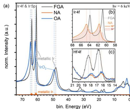
The IrO<sub>2</sub> electrode remains chemically stable for annealing in oxygen atmosphere. For annealing in nitrogen atmosphere, a chemical reduction of the IrO<sub>2</sub> electrode starts and results in metallic Ir layer on top of the IrO<sub>2</sub> electrode. Finally, forming gas annealing causes a complete reduction of the IrO<sub>2</sub> top electrode into metallic Ir.
