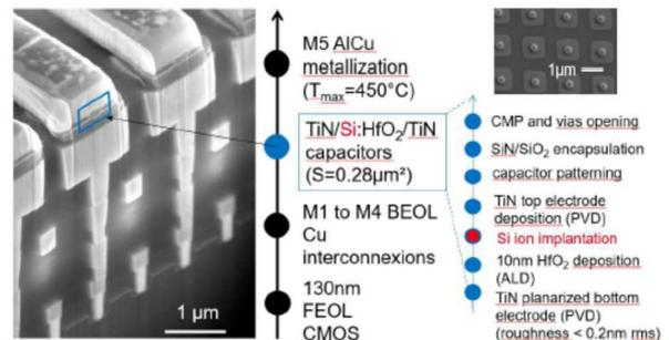
10 nm Si-implanted HfO<sub>2</sub> is demonstrated to be ferroelectric for the first time when integrated in a Back-End-Of-Line (BEOL) 130 nm CMOS. Scaled 0.28µm<sup>2</sup> capacitors demonstrate excellent endurance (10<sup>9</sup> cycles measured at 4V, extrapolated to be 10<sup>12</sup> at 3V), with tight coercive field distributions at wafer scale and excellent data retention at 85°C.
