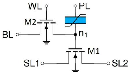
A second transistor M3 is the read transistor that is used to monitor the potential of floating node n1 during read operation by measuring its S/D current via SL1. Finally, the PL connects to the second terminal of the ferroelectric capacitor.
