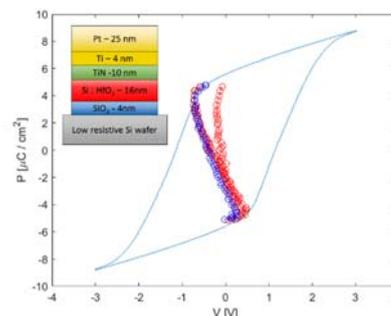
Work at the Ecole Polytechnique Fédérale de Lausanne has demonstrated negative capacitance in a FeFET like geometry using a Si/SiO<sub>2</sub>/Si:HfO<sub>2</sub>/TiN structure. The NC shows up only at short (ns) pulses (and destroyed by dc). With faster pulses and thicker SiO<sub>2</sub> layers one can expect a stronger NC and lower level of leakage. Further enhancement of the NC may require more stable polarization without multidoman formation.
